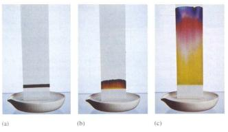
Paper chromatograph of ink. (a) A line of the mixture to be separate is placed at one end of a sheet of porous paper. (b) The paper acts as a wick to draw up the liquid. (c) The component with the weakest attraction for the paper travels faster than those that cling to the paper.
